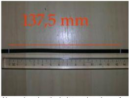
Always keeping the belt taped on the surface, take two marks with a marker at a distance of 137,5mm one to each other. It's not important where you draw the first mark, but it's fundamental that the second is drawed at 137,5 mm from the first.
