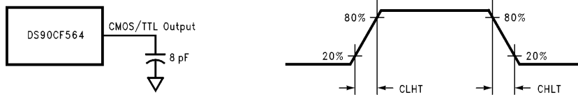
FIGURE 4. DS90CF564 (Receiver) CMOS/TTL Output Load and Transition Times
