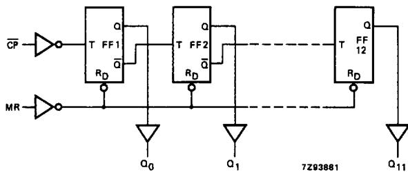
Fig.5 Logic diagram.
