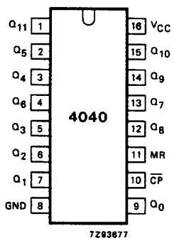
Fig.1 Pin configuration.
