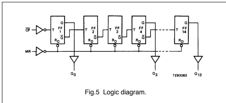
Fig.5 Logic diagram.
