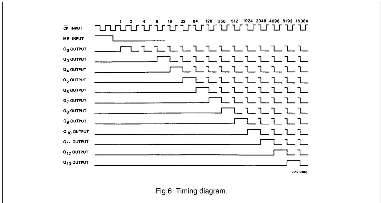
Fig.6 Timing diagram.
