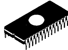
CERAMIC PACKAGE DIP-28C-C01
